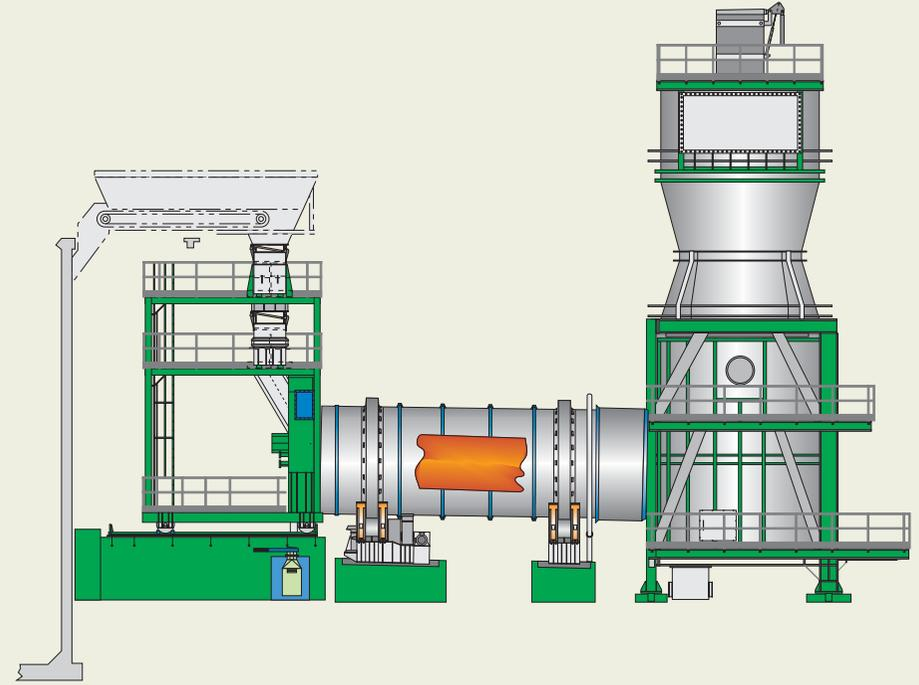
Rotary kiln plant with afterburner chamber
