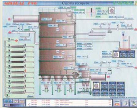
In case of powdery dust or increased temperature at the bottom of the boiler in spite of low frequency vibrators the ultrasound cleaners are activated. The ultrasound cleaners, too, are regulated by an operation – break time control system providing for a periodical cleaning of this part of the boiler.
