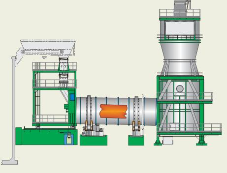
Rotary kiln plant with afterburner chamber
